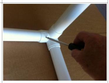
Insert the (2) special screws into the pre-drilled holes on the insides of the top two bars.
